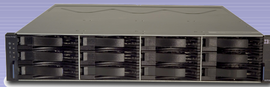
IBM System Storage DS3200 SAS host interface disk system
